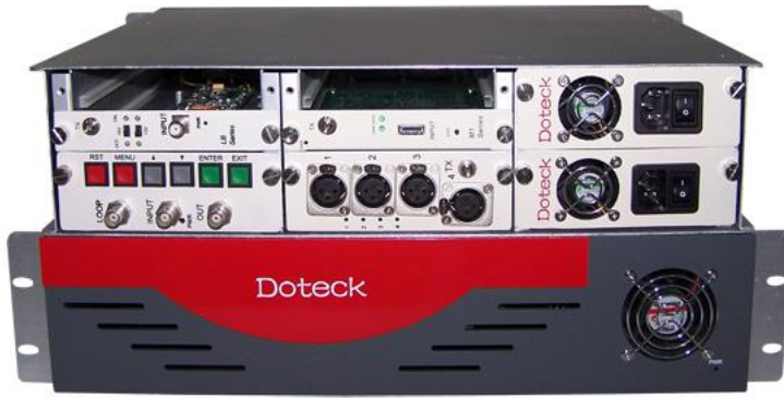
8-slot, 19-inch, dual power supply
